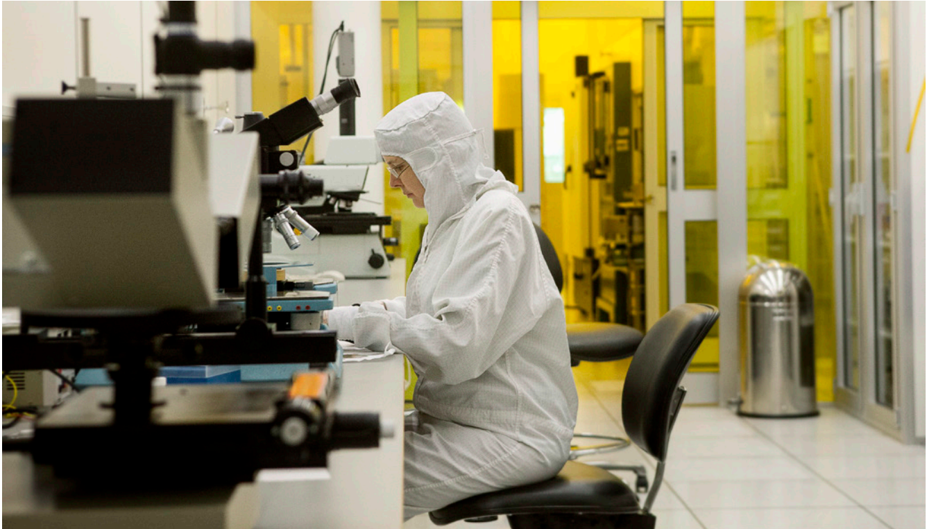
Dust-free cleanrooms are essential when manufacturing sensors and other sensitive electronics. Magnus Berggren's laboratory in Norrköping.
