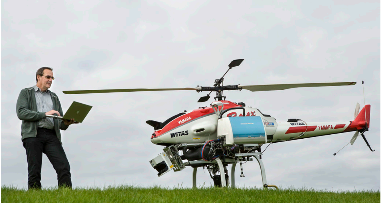
In the WITAS project, a helicopter was constructed that could maneuver in the air without a pilot. This photo shows Patrick Doherty with the unmanned helicopter.
