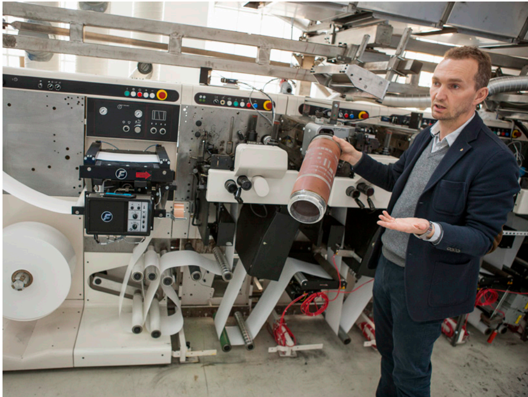
An ordinary printing press has been repurposed to print electronic components on paper. Electronic ink is put into the containers that would normally hold printer's ink. Magnus Berggren demonstrates.
